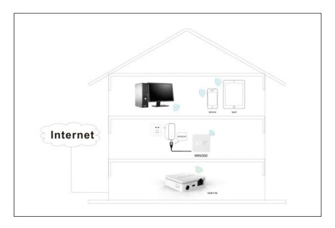
2. Intelligent WiFi Bridge mode(MINI300): WiFi intelligent bridge function, wireless to wired, wired to wireless intelligent switching
